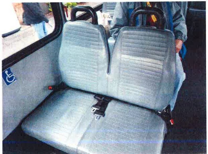
Figure 4. Notchback Effect Foldaway Seat Design
