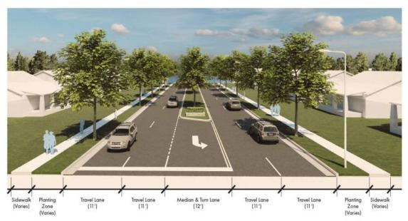
Figure 86 includes gateway signage, four 11' travel lanes, a 12' median and turn lane, and an activated curbside with a planting zone and sidewalk.
