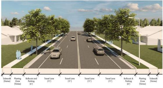
Figure 87 includes four 11' travel lanes, with bulbouts and parking separating the travel lanes from the planting zone and sidewalk.
