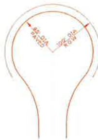
Figure D103.1 DEAD-END FIRE APPARATUS ACCESS ROAD TURNAROUND
