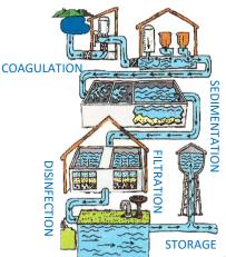
Next, the slow flow through the sedimentation basin allows the heavier particles to settle out. Sedimentation removes the majority of the sediment from the water.
